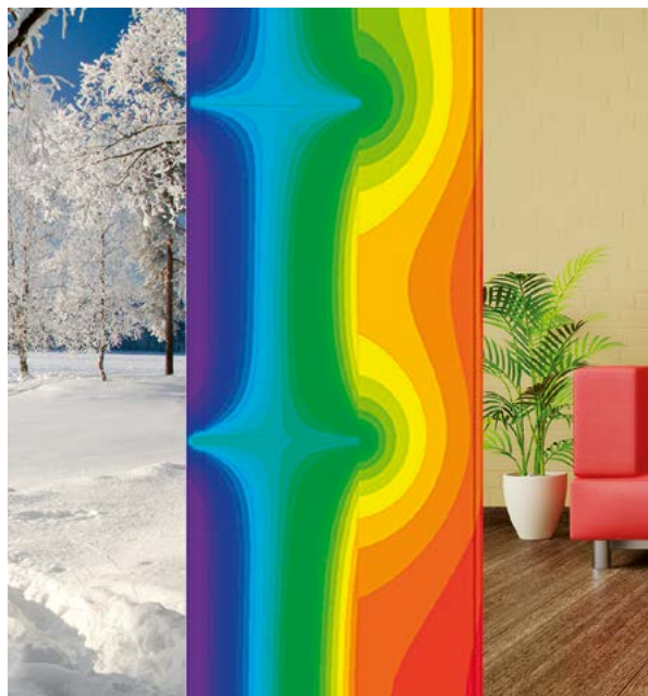
Image 1 Pronounced thermal bridge on aluminum consoles
